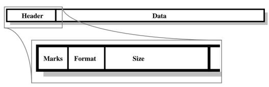
The header contains mark bits (the same as in unboxed words), a code indicating the format of the data section, and a size (number of items in the data section).
