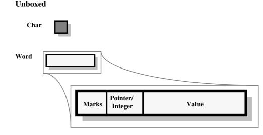
Unboxed words are further structured. They contain mark bits (used by the garbage collector and the persistence mechanism), a flag indicating whether this is an integer or a pointer (again, needed by the garbage collector), and an integer or pointer value.
