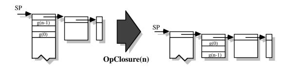
Recursive and mutually recursive functions need recursively defined closures. These are built in two steps, first allocating empty closures and later filling them. **OpDumClosure(n)** builds dummy closures of n globals, given a text object on the stack.
