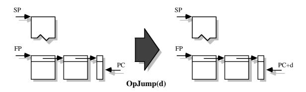
Conditional jumps are obtained by the **OpTrueJump(d)** and **OpFalseJump(d)** instruction, where d is a relative displacement from the current PC. Again, the exact meaning of d depends on implementations. OpTrueJump jumps if the top of the stack has the value true in it, otherwise proceeds to the next instruction. In both cases the top value is popped away. The following picture shows the two transitions for OpTrueJump; OpFalseJump is symmetric.
