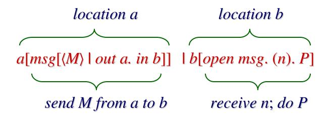
The packet msg moves from a to b, mediated by the capabilities out a (to exit a), in b (to enter b), and open msg (to open the msg envelope).
